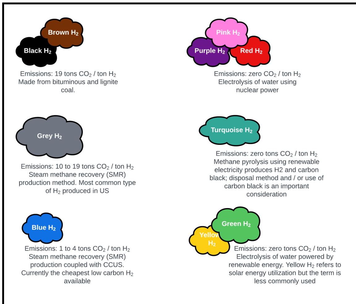
Figure RB1. “Colors” and associated CO 2 emissions for hydrogen produced by various methods.
